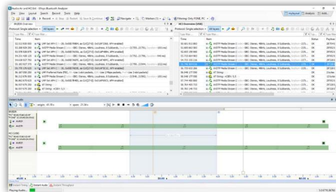
Audio captured over HCI or from an Audio I2S input [PRO] can be played back as well. This enables characterization of the complete audio chain, from the uncompressed audio provided to the source radio chip, to the audio transmitted wirelessly, and the decoded audio received by the receiver radio chip. The various audio streams are exportable to WAV format.
